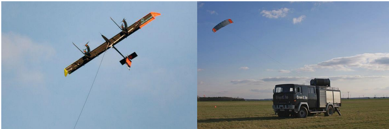
The concepts in real life: Google's Makani flying wind turbine on the left, and a soft-kite yoyo configuration from German competitor Enerkite. The drum can be seen on the top of the truck. The flying is autonomous, the driving not.
