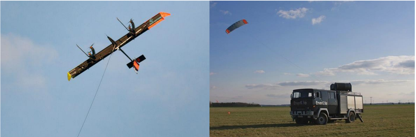
The concepts in real life: Google's Makani flying wind turbine on the left, and a soft-kite yoyo configuration from German competitor Enerkite. The drum can be seen on the top of the truck. © Google Makani, Enerkite
